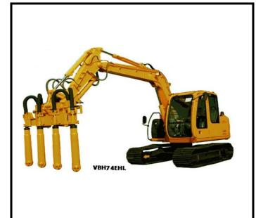
When mass-placement of concrete is required there is no greater labor savings tool than VIBACK. The unique hydraulic vibrator design yields maximum concrete consolidation and compaction, ideal for dam construction job sites. Available as a complete base machine or "attachement" to use on existing base machines.
