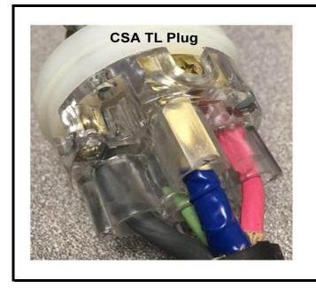
The <u>CSA TL (Twist Lock) Plug</u> is a 5 pin grounding type plug. The HBM CSA Series vibrators have a specific wiring configuration using the center ground pin. Green Wire to "Center Pin" White Wire with Blue Mark to "Y" Black Wire to "X" Red Wire to "Z"
